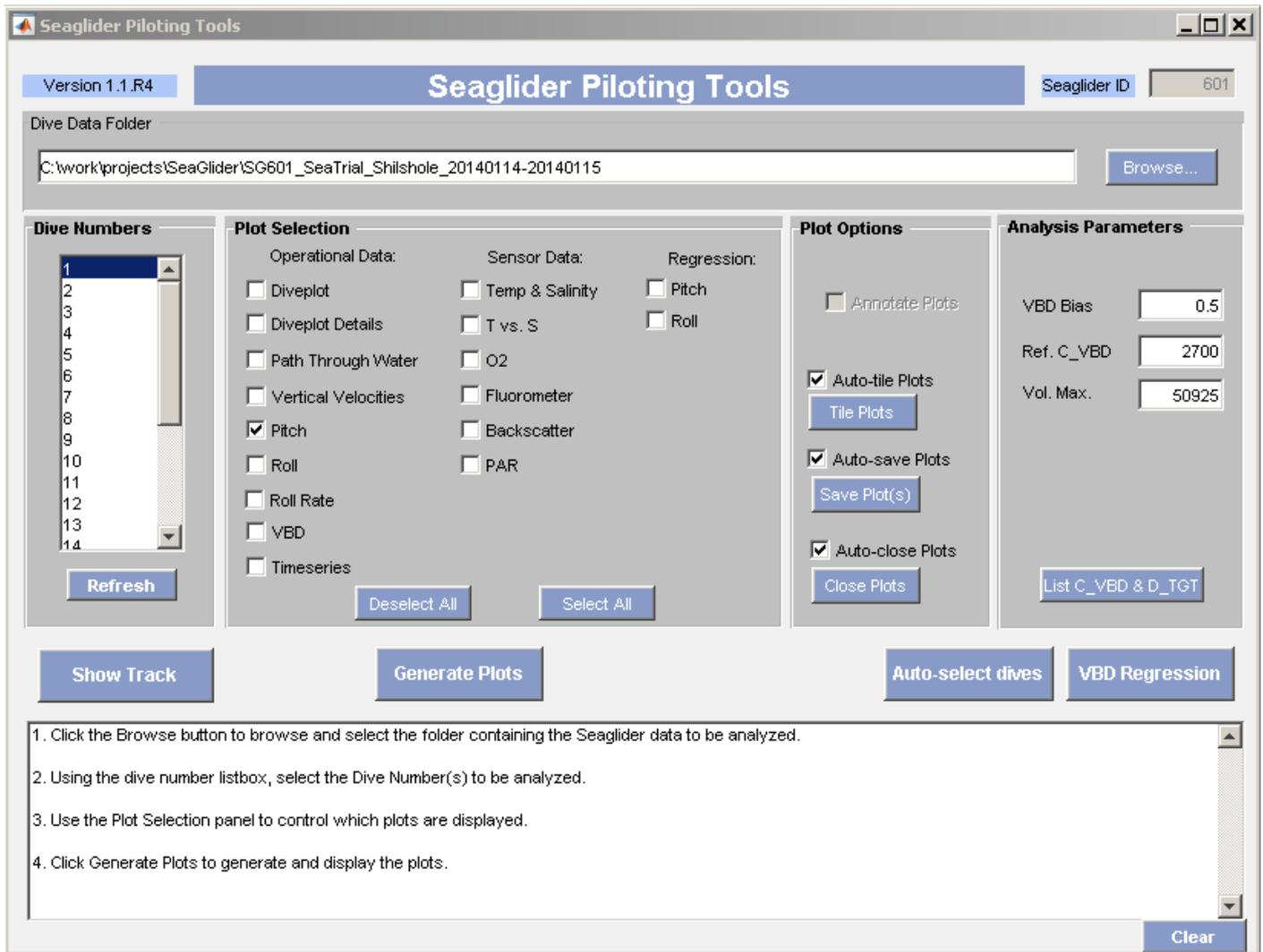
Figure 3 Piloting Tools window
