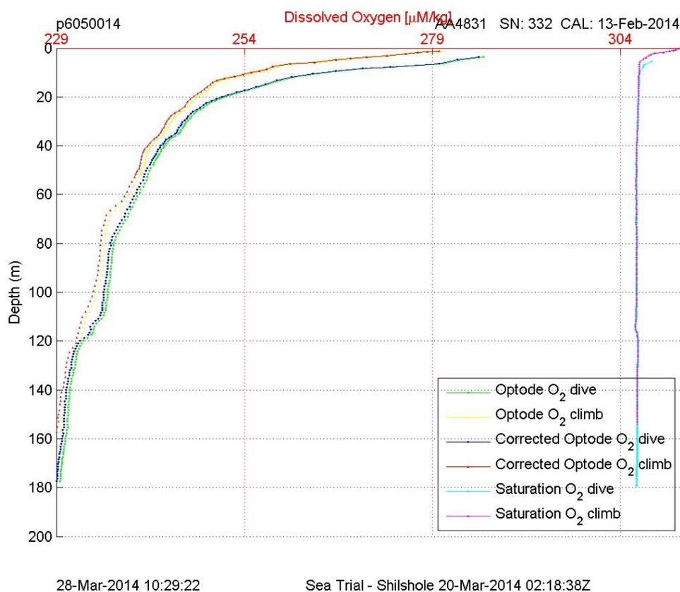
Figure 15 Dissolved Oxygen plot
