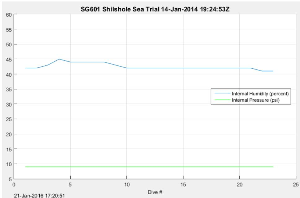
Figure 19 Internal Humidity & Pressure plot
