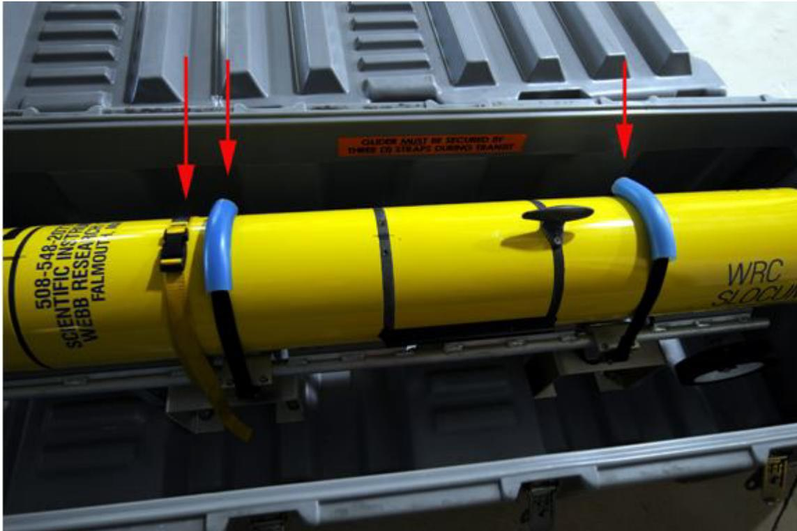
Ensure that all three straps are secure (two crate straps and one cart strap). If extra supplies are included in the crate, ensure that they will not interfere with the fin or become dislodged during transit.
