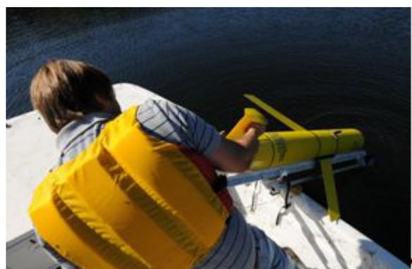
Lower the cart into water, and manipulate the glider by the digifin into position on the cart. Lift and tilt the glider onto the ship's deck.
