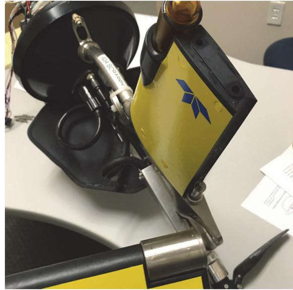
**Figure 1-16 The Rudder Removed from Tail Fin**
