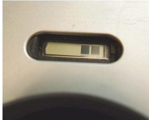
**Figure 1-11 Battery Charge Indicator Bars**
