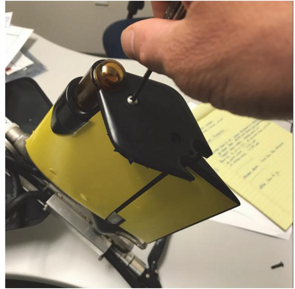
**Figure 1-14 Removing the two Phillips Head Screws**
