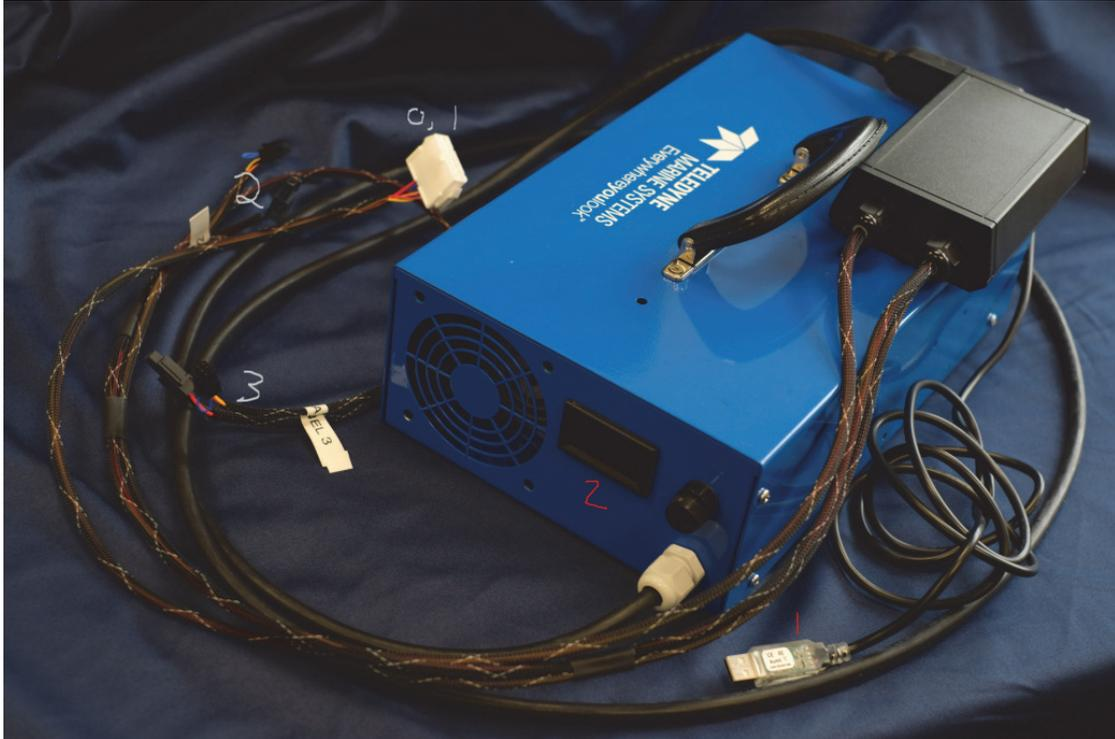
**Figure 1-8 Battery Charger with Charging Cable**
