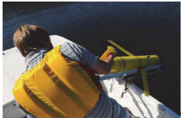
Lower the cart with nose ring into water, and manipulate the glider by the tail boom into position on the cart. Lift and tilt the glider onto the ship's deck.
